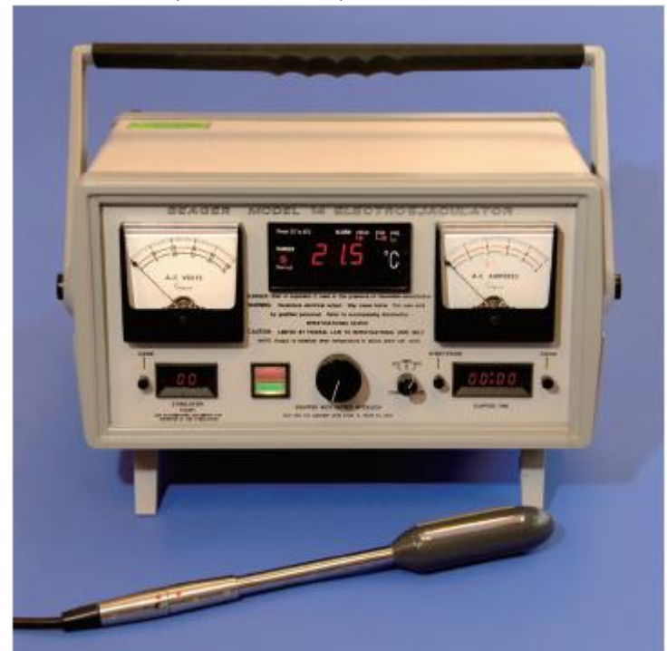
Figure 3: Electroejaculation machine with an attached rectal probe.
